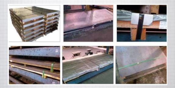
• Plates larger than 16.0 mm: should be supported by wooden chicks and strapped;
